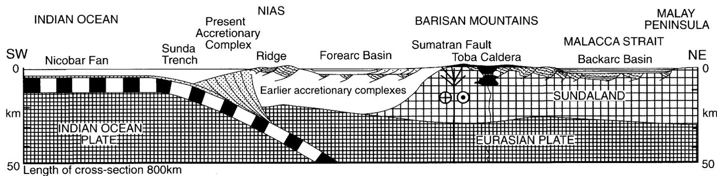
Fig. 1.3. Diagrammatic section across the Sumatran Subduction System from the floor of the Indian Ocean to the Malay Peninsula, drawn to scale.
