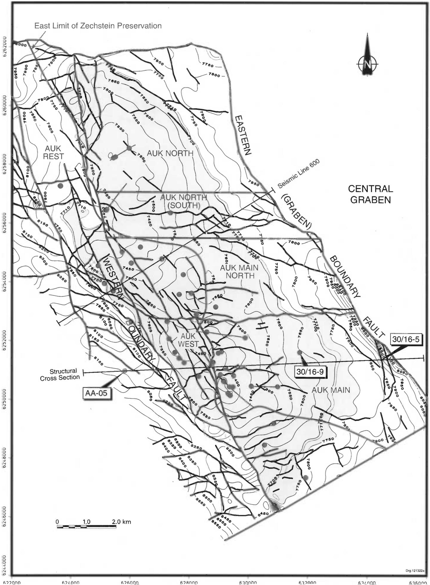
**Fig. 2.** Top Rotliegend structure map and well locations. The Zechstein is only preserved in the west part of the field, towards the east Early Cretaceous erosion has removed all of the Zechstein and cut into the Rotliegend reservoir.
