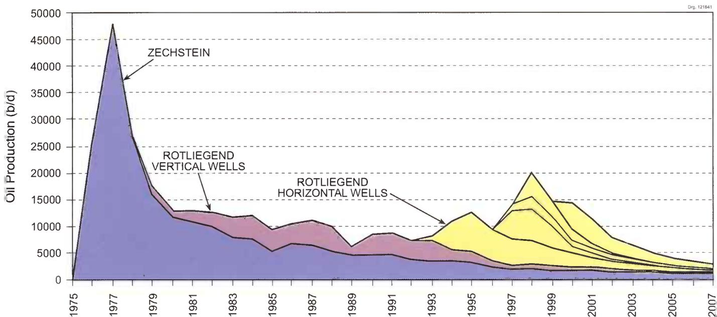
**Fig. 11.** Production contribution of the individual reservoirs and well types in the Auk Field. Note that the amount of oil produced from Zechstein wells includes cross-flow from the Rotliegend reservoir.
