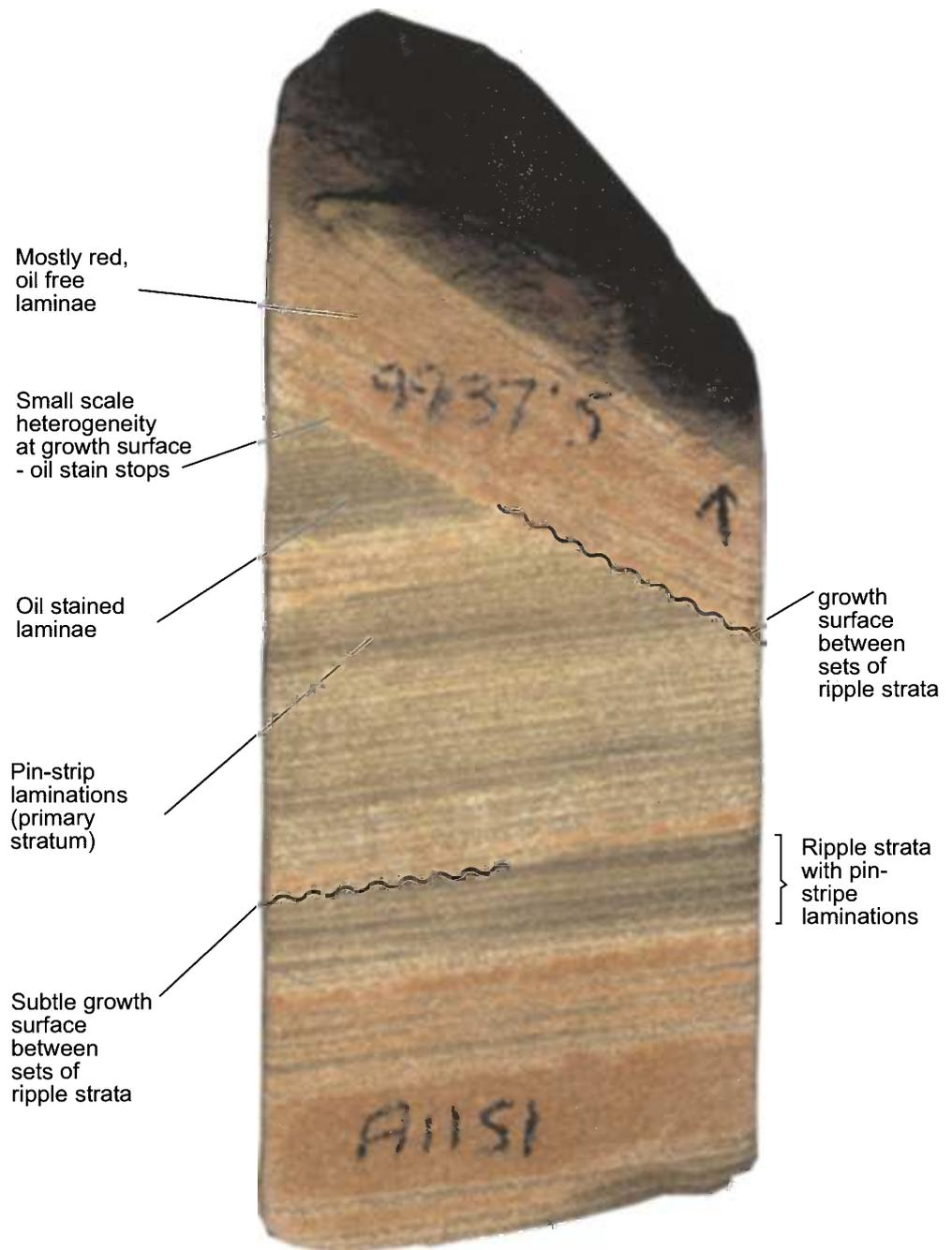
**Fig. 8.** Example for lithofacies identification in cores. Note fine scaled intercalations of oil stained (brown) and oil free reservoir (red).
