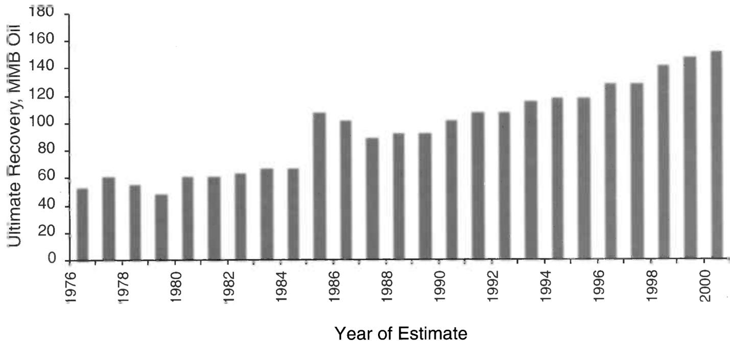
**Fig. 10.** Changes of reserves estimates in the Auk Field were dictated by early water-break-through (1979), plans for installation of artificial lift (1985–1988), and horizontal well and seismic imaging technology (1990s).
