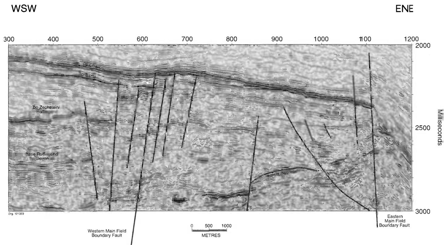
**Fig. 4.** Seismic cross-section in SW–NE direction through the Auk Main North block. The quality of the 1991 3D seismic survey in the latest reprocessing, shown in this figure, is now sufficient to interpret reservoir juxtapositions reliably.
