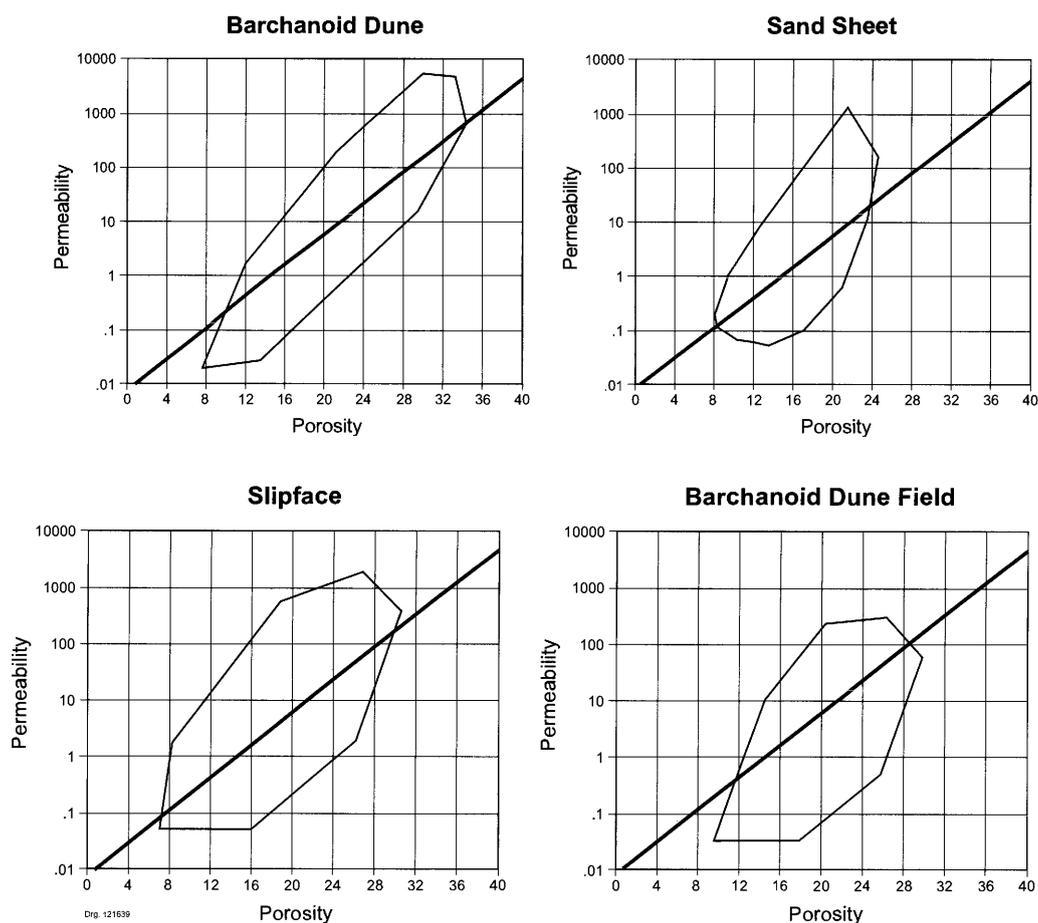
**Fig. 6.** Porosity/permeability relationship for the different lithofacies in the Rotliegend unit 2 main reservoir. The permeability rarely exceeds 1000 mD, in barchanoid dunes.
