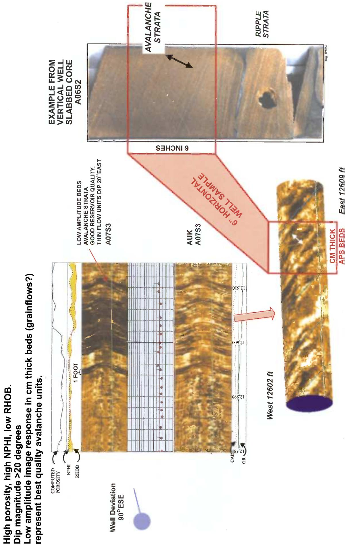
Fig. 9. Identification of avalanche strata in UBI images of a horizontal well. See Follows (1997) for full description of core/UBI log interpretation in this well.
