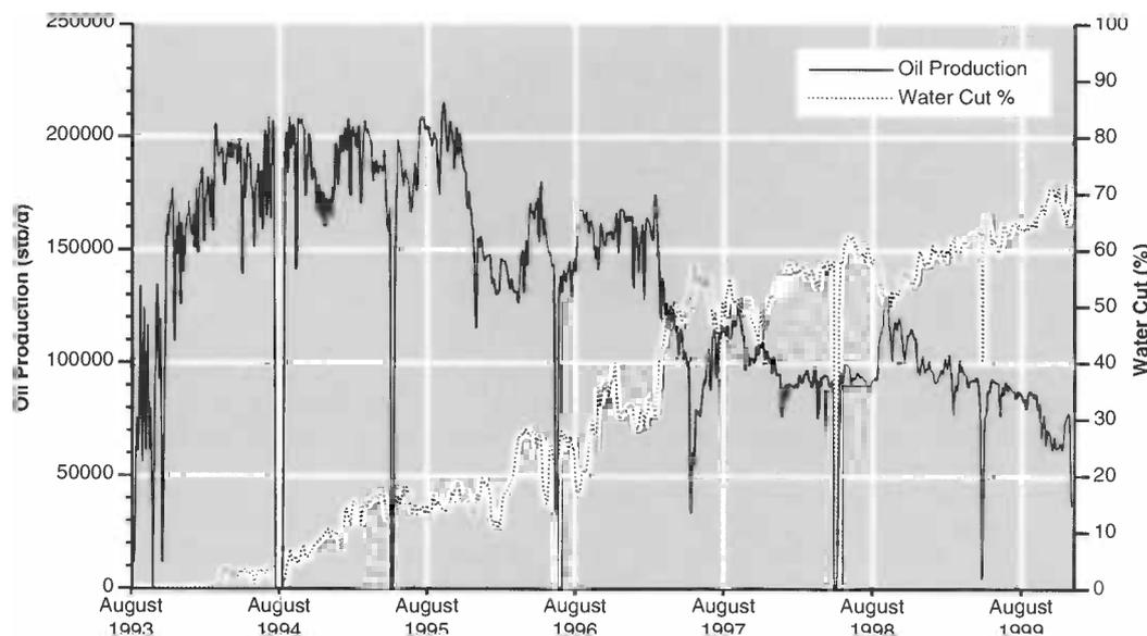
**Fig. 14.** Oil production plotted against time since first oil. Also shown is the percentage water cut since water breakthrough. Major decreases in oil production correspond to the watering out of key reservoir intervals during field life. Typically oil production from wells declines rapidly once they have cut water.
