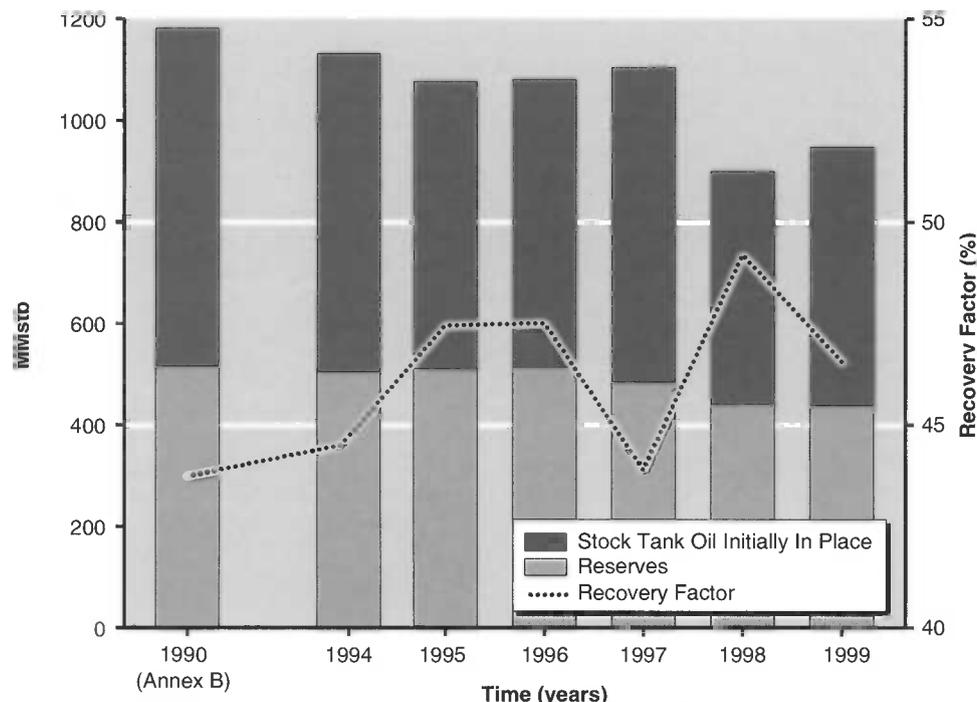
**Fig. 15.** Scott Field STOIP, reserves, and recovery factor plotted against time. The first column shows data from the Scott Field Annex B in 1990. Subsequent columns show data from annual field reports since first oil in September 1993. Since the Annex B there has been a 20% decrease in field STOIP, and a commensurate 14.5% decrease in field reserves. Over the same period, the projected recovery factor from the field has increased.
