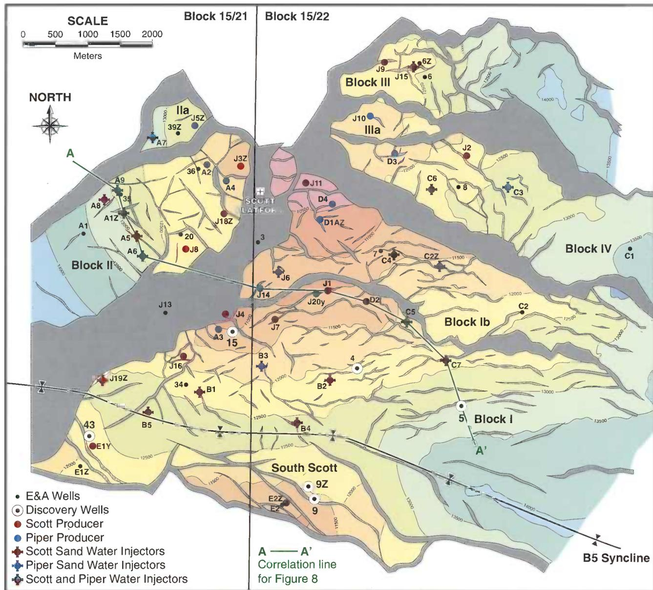
Fig. 3. Top Piper Formation structure map for the Scott Field showing the location of exploration, appraisal and development wells.
