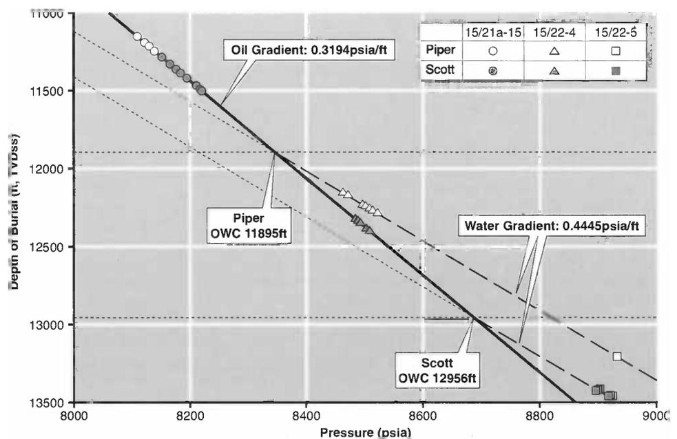
Fig. 4. Reservoir fluid pressure data for exploration wells 15/22-4, 15/22-5 and 15/21a-15. Data shows oil and water pressure gradients in the Scott Field structural Block I and the inferred oil-water contacts in the block. Note that the oil-water contact in the Piper Sandstones is significantly shallower than that in the Scott Sandstones, creating a perched contact.
